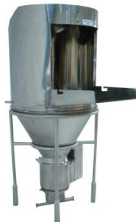
FlexiSieve™ under a sack opening station. Note. Vacuum Transfer pick up under FlexiSieve™
